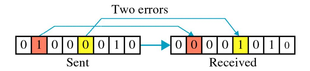
The term **burst error** means that two or more bits in the data unit have changed from 1 to 0 or from 0 to 1.
