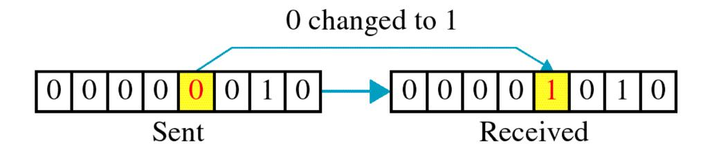
Single bit errors are the least likely type of errors in serial data transmission because the noise must have a very short duration which is very rare. However this kind of errors can happen in parallel transmission.
